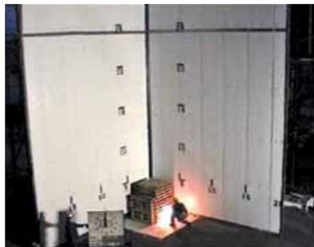
Set up of FM full scale fire test prior to commencement (Note the use of a large wooden crib as the fire source).
