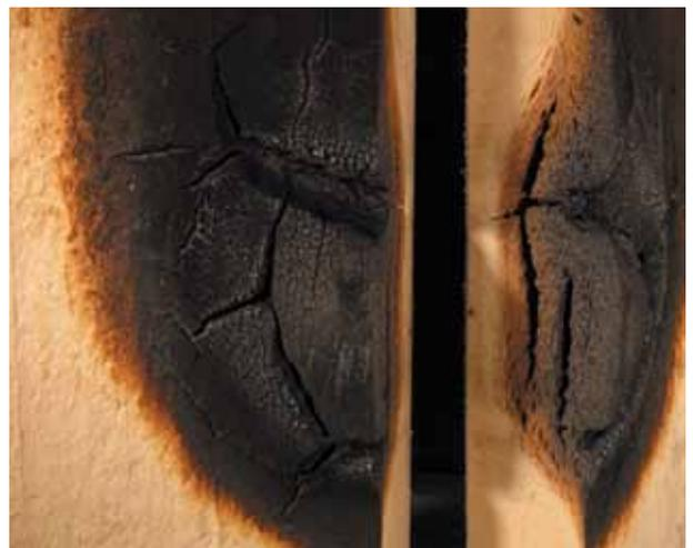
*Section cut through the Kingspan PIR panel showing no fire propagation after 30 minutes*
