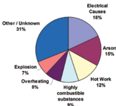
Many of these causes are difficult to predict or control, and therefore panel systems with material cores that offer poor fire performance will always present some level of risk in the event of a fire.
