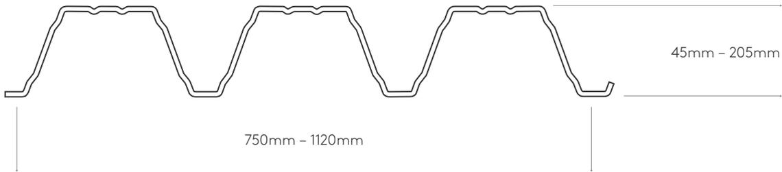
Please note: all Structural Liner Deck profiles can be perforated in the web.
